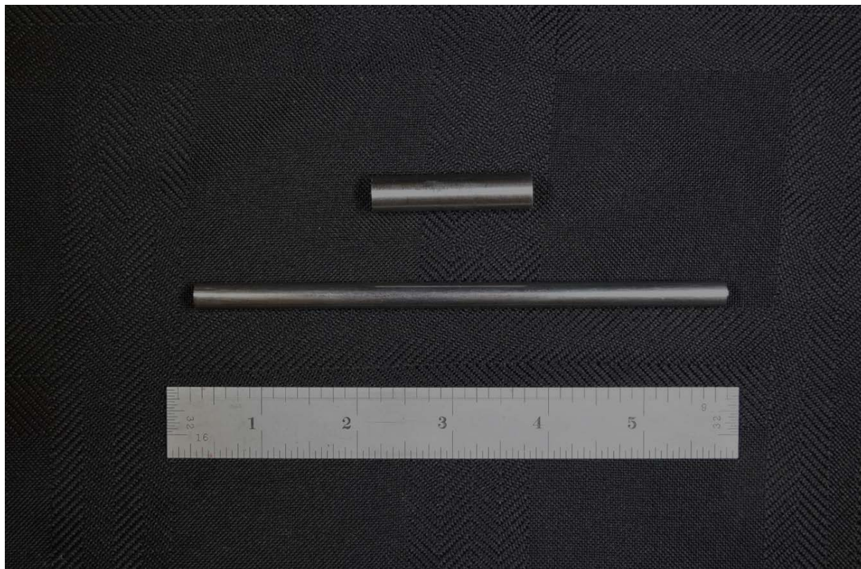
Figure 5.3. Photograph Showing 304 Stainless Steel Tube with Starting Thick-Wall Tube (top) and Finished Thin-Wall Tube (bottom)
