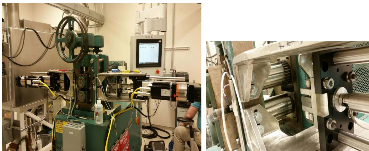
Figure 2.1. Modifications to the PNNL Rolling Mill for Lab-Scale Pilgering
