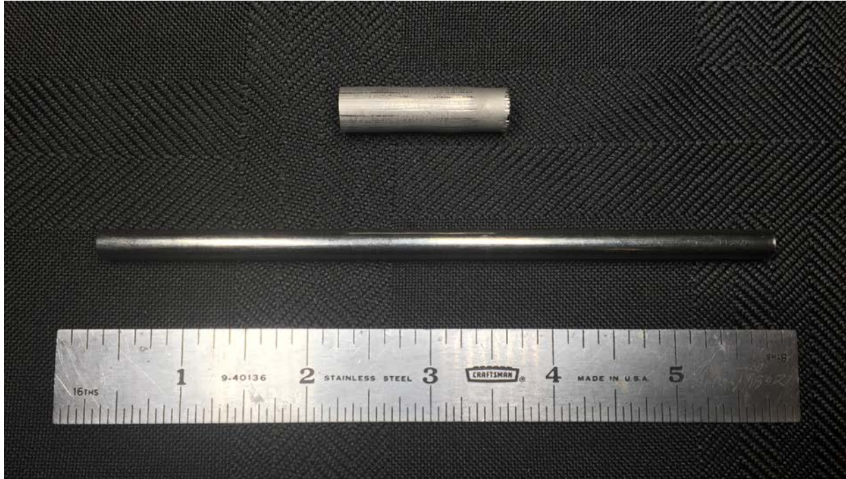
Figure 5.6. Photograph Showing 14YWT Starting Blank (top) with Finished 14YWT Thin Wall Tube (bottom)
