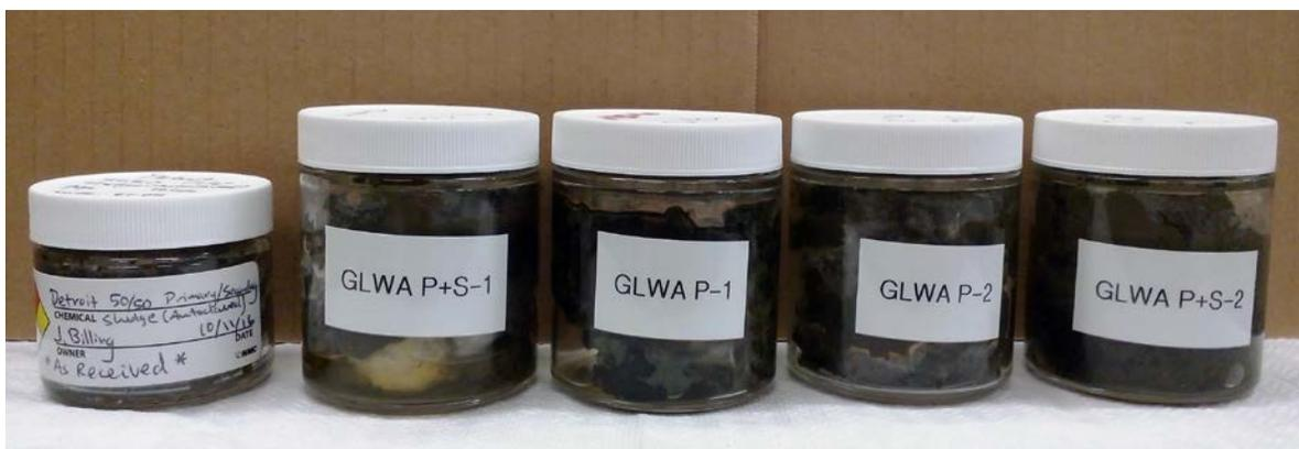
**Figure 1.** Sludge samples used for PPCP and PFC extraction.
