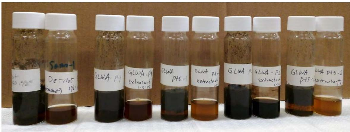
**Figure 2.** Sludge extracting vials after centrifugation (left) and vials with separated extractant (right).
