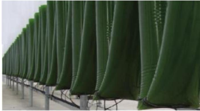
**Figure 2.1.** Vertical Plastic Bag PBR Example (Huang et al. 2017)
