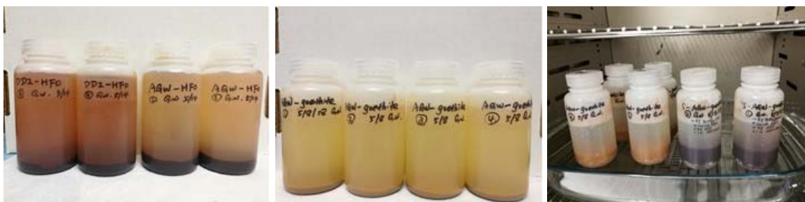
Figure 5.1. Iron oxides [HFO (left) and goethite (middle)] preparation in polyethylene vessels; the conversion of AGW-HFO to AGW-goethite (right) was visible by color changing, where no obvious color changed in the SAGW systems, indicating the conversion of HFO to goethite was strongly retarded when sediment was included.
