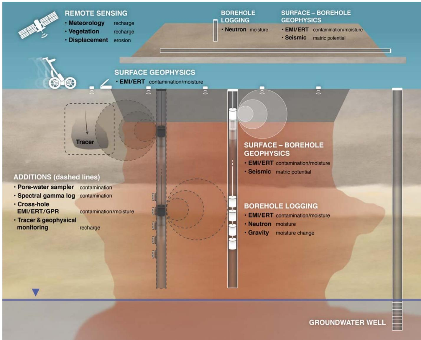
**Figure 16.** Conceptual depiction of the monitoring components for a surface barrier remedy configuration.
