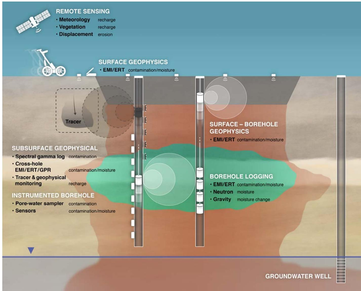
**Figure 17.** Conceptual depiction of the monitoring components for an in situ remedy configuration.
