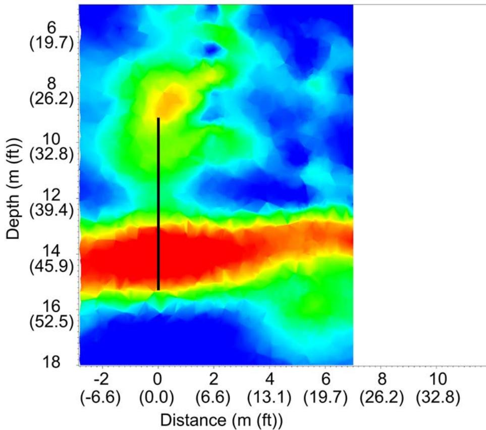
**Figure 11.** Image of bulk EC for the Hanford soil-desiccation DVZ treatability test using cross-borehole ERT.
