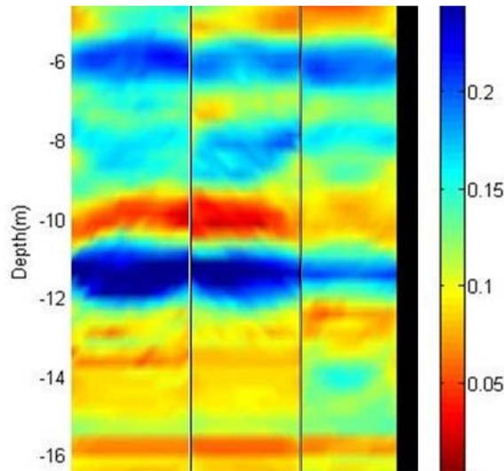
**Figure 10.** Image of EM velocity for the Hanford soil-desiccation DVZ treatability test using cross-borehole GPR.
