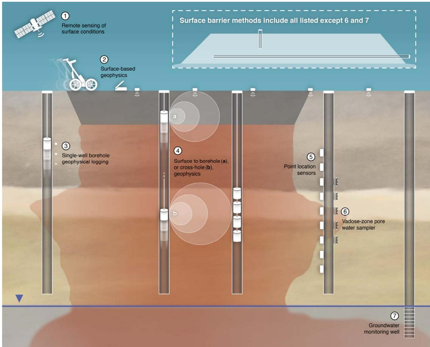
**Figure 5.** DVZ monitoring methods. Numbers shown inside white circles correspond to the numbered monitoring methods in Table 1.
