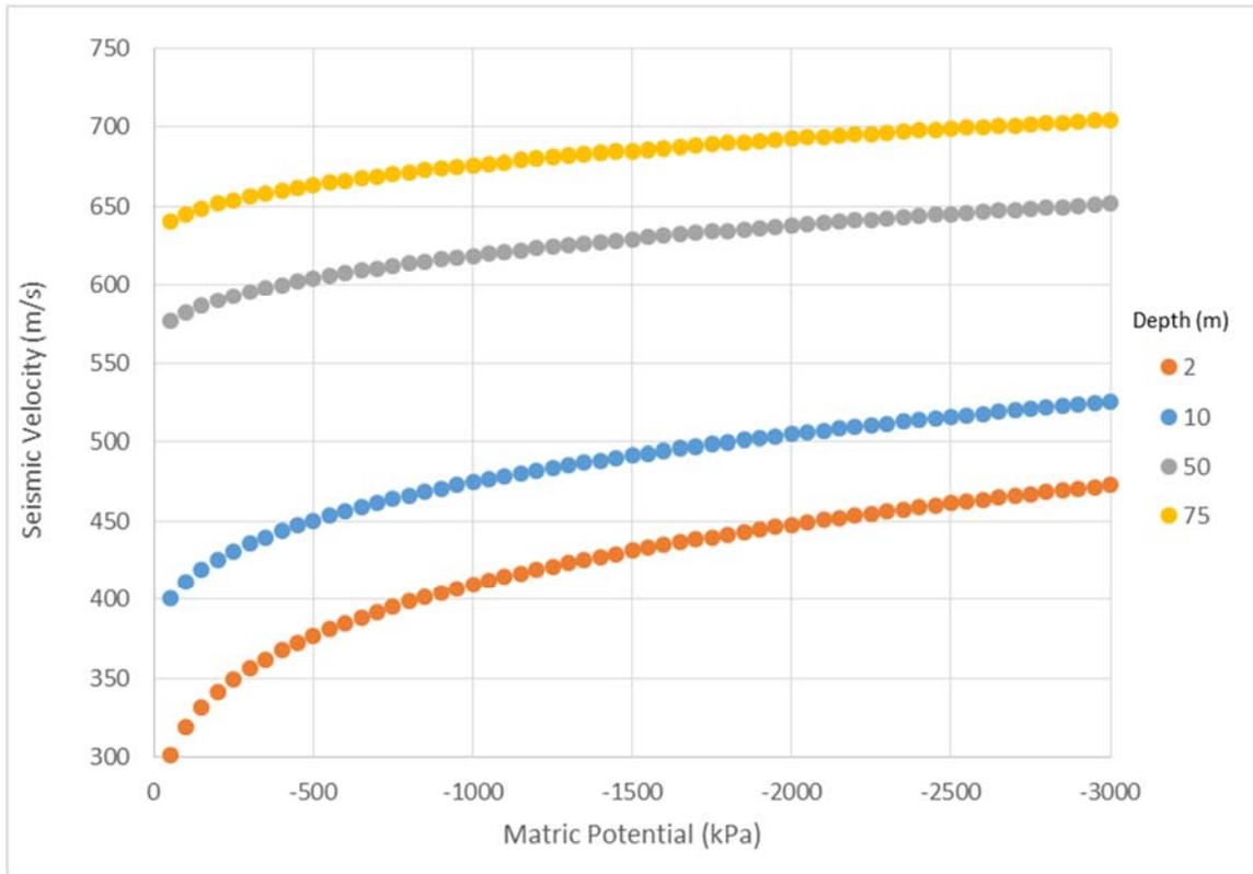
**Figure 12.** Functional relationship illustrating the dependence of seismic velocity on overburden depth/stress and matric potential at depths of 2, 10, 50, and 75 m.
