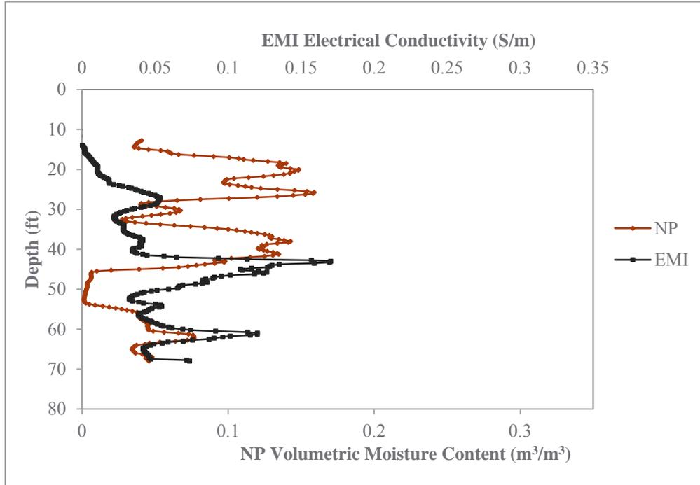
**Figure 13.** EMI and neutron probe single borehole logs from the soil desiccation DVZ treatability test.
