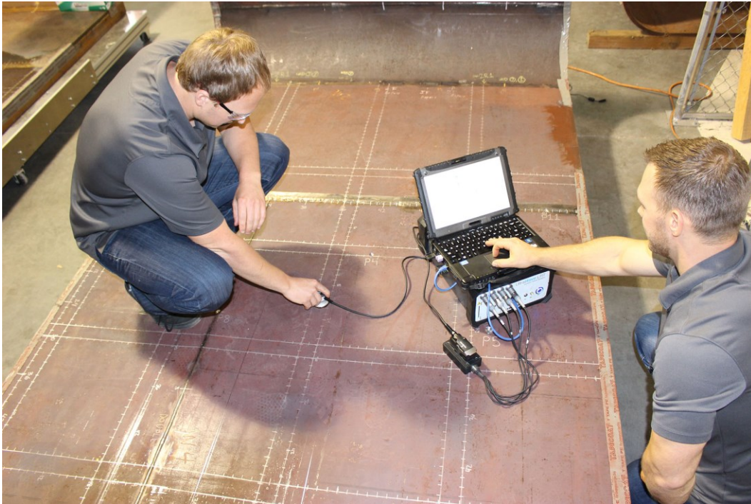
Figure 6. GWP Sensor Inspection Locations on the 1/2-inch-thick Bottom Plate of the SET Mock-up during the FY 2017 Phase I test campaign Sensor Effectiveness Testing
