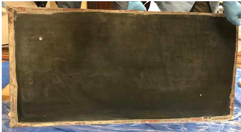
Figure 8. Bottom of the Test Plate after Removing the Slurry, Revealing the Two Locations of the Pits
