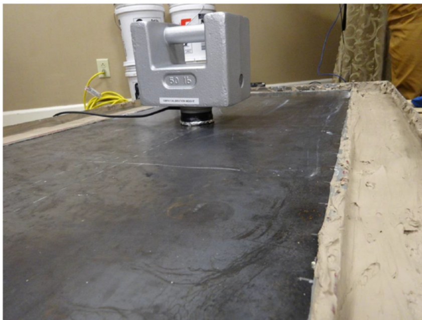
Figure 2 Photograph of the GWPA probe under the dry-coupling configuration with the coupling membrane and the 50-lb calibration weight present.
