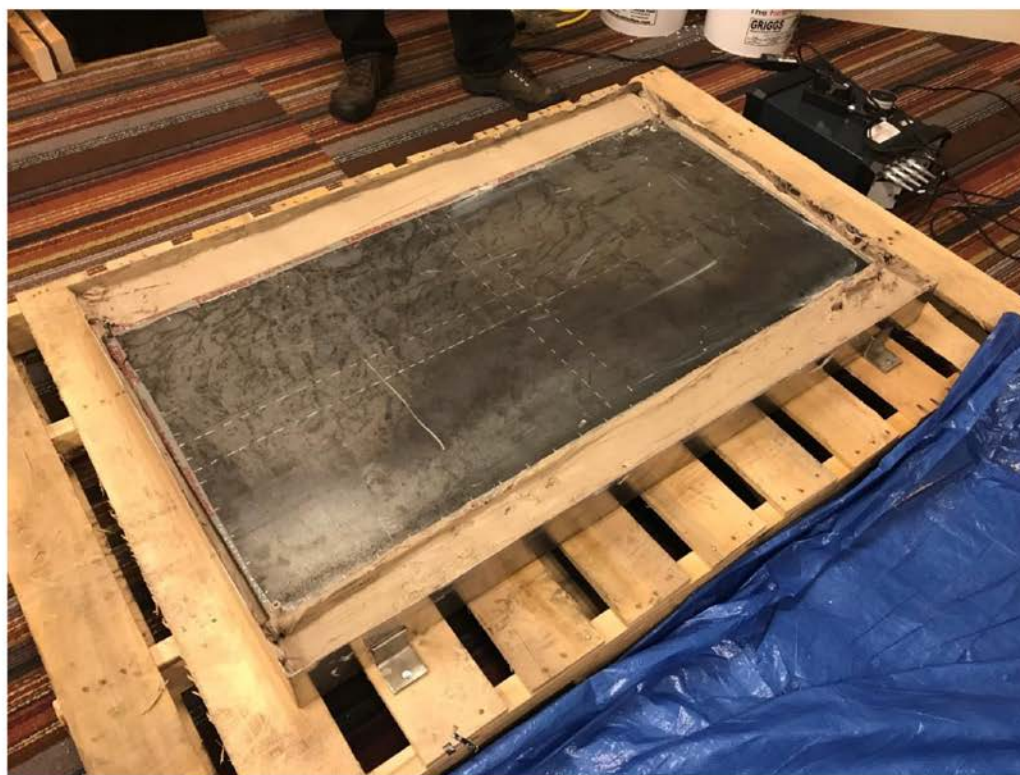
Figure 1 Photograph of the test plate in the slurry with the GWPA system on the left.
