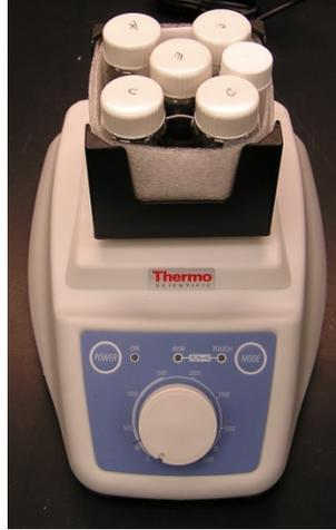
**Figure 2.2.** Thermo LP Vortex Mixer with Retrofitted Vial Holder for In-Cell Sample Batch Contact Shaking
