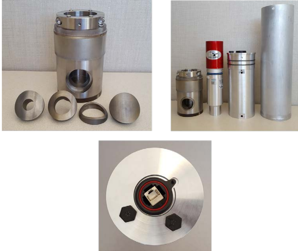
Figure 18. Tungsten collimator with inserts of varying aperture diameter: 2 cm, 3 cm, 4 cm, and full plug (top left), detector assembly (top right), and dual liquid-tight air vents along with sealed Power over Ethernet (PoE) port equipped with collimator aligning notch (bottom).
