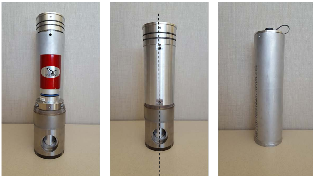
Figure 19. Detector assembly out of the aluminum enclosure (left), notch-aligned aluminum spacer with dual O-ring top-cap (center), and fully assembled detector module (right).
