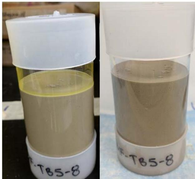
**Figure A.5.** Free liquid photos for TB5 (Simulant 5, Cast Stone) on the day of production (left) and three days after production, when no free liquids were observed (right).
