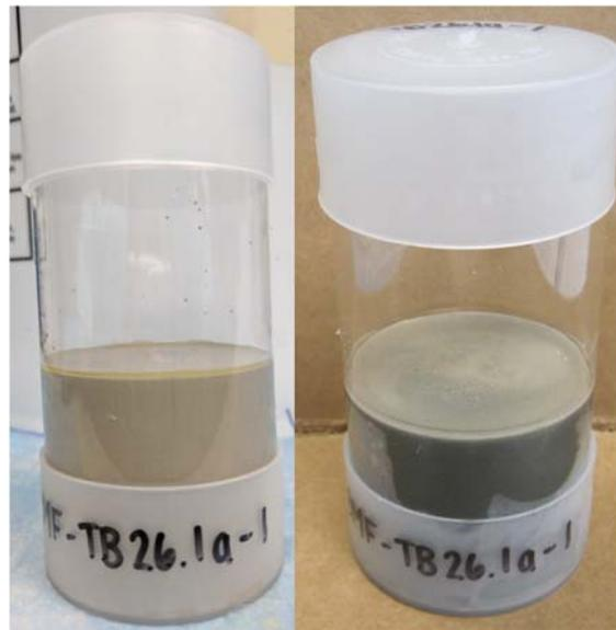
**Figure A.27.** Free liquid photos for TB26.1a (Avg simulant, 10% HL, 18% OPC, 72% BFS) on the day of production (left) and 8 days after production, when <1 vol% free liquids were observed (right).
