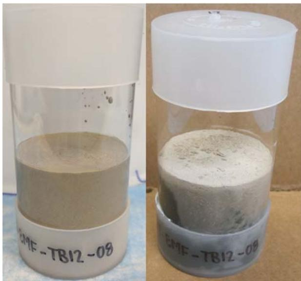
**Figure A.12.** Free liquid photos for TB12 (Simulant 4, Aquaset/BFS) on the day of production (left) and 18 days after production, when no free liquids were observed (right).
