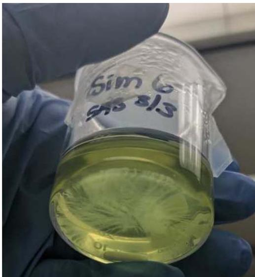
**Figure 3.1.** Simulant 6 Precipitate after Heating at  $\sim 50^{\circ}\text{C}$  for Several Hours
