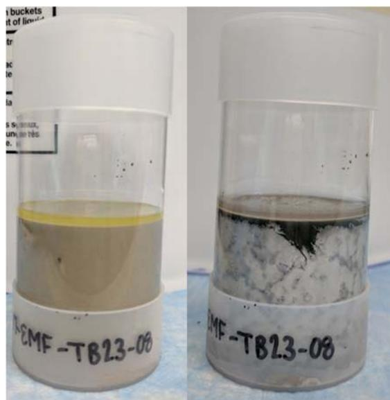
**Figure A.23.** Free liquid photos for TB23 (Simulant 7, OPC/BFS) on the day of production (left) and 12 days after production, when  $<1$  vol% free liquids were observed (right).
