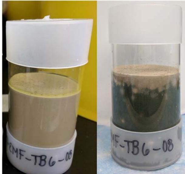
**Figure A.6.** Free liquid photos for TB6 (Simulant 6, Cast Stone) on the day of production (left) and five days after production, when no free liquids were observed (right).
