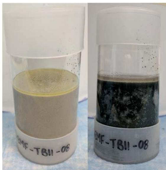
**Figure A.11.** Free liquid photos for TB11 (Simulant 3, Aquaset/BFS) on the day of production (left) and 18 days after production, when  $<1$  vol% free liquids were observed (right).
