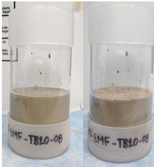
**Figure A.20.** Free liquid photos for TB20 (Simulant 4, OPC/BFS) on the day of production (left) and 4 days after production, when no free liquids were observed (right).
