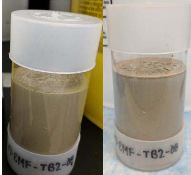
**Figure A.2.** Free liquid photos for TB2 (Simulant 2, Cast Stone) on the day of production (left) and three days after production, when no free liquids were observed (right).
