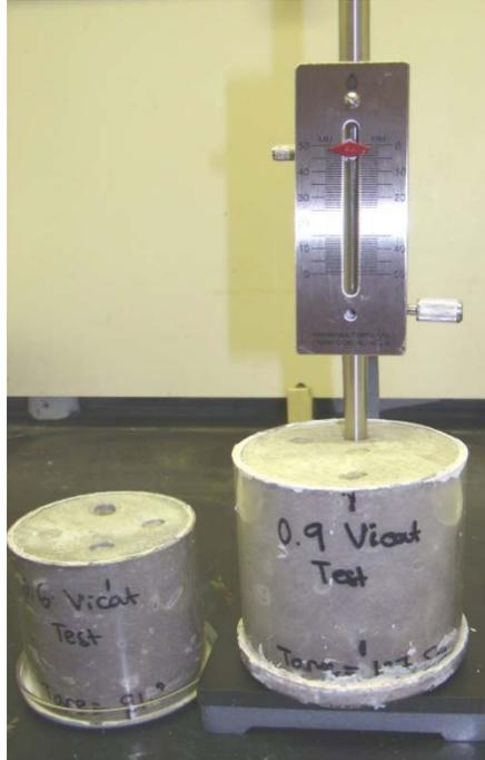
**Figure 5.1.** Vicat Needle Apparatus Showing Complete Penetration of the 1 mm Diameter Needle Such That the Rod Has Made an Indentation in the Specimen Surface in Previously Tested Areas. The sample shown is not associated with the samples discussed in this report.
