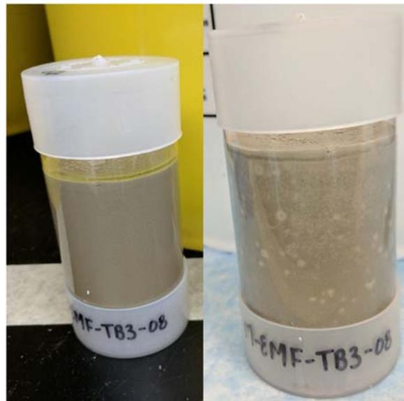
**Figure A.3.** Free liquid photos for TB3 (Simulant 3, Cast Stone) on the day of production (left) and three days after production, when no free liquids were observed (right).
