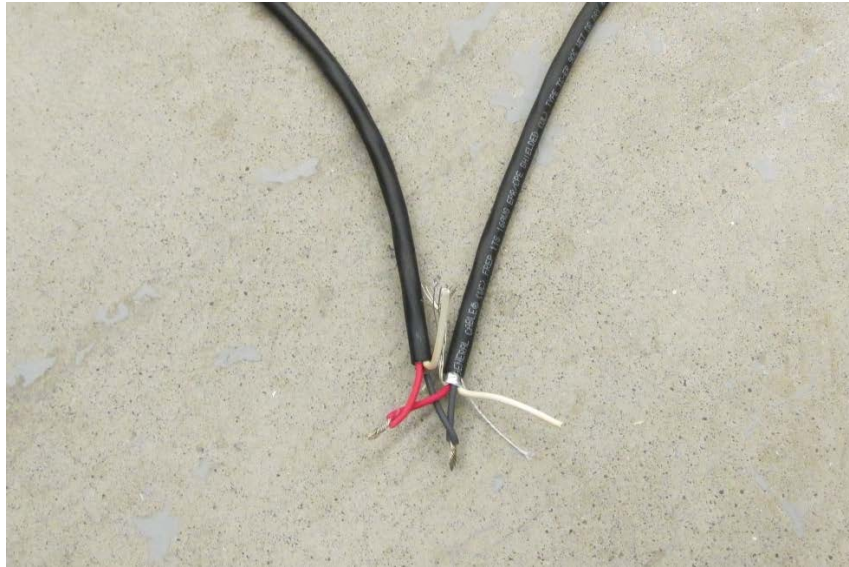
Figure 9.50. Twisted wire connections made between 10 ft. extension cable and the 100 ft. three-conductor shielded cable under test.
