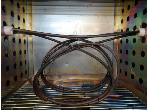
Figure 9.13. Aged cable configurations for (left) in-situ LIRA measurements and (right) ex-situ VNA measurements.
