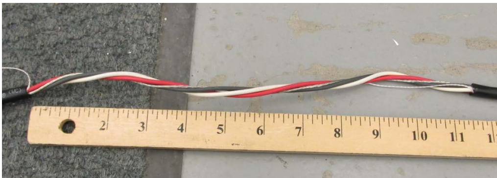
Figure 9.47. Mechanical defect consisting of 12 in. section of removed jacket and shield along the three-conductor shielded cable
