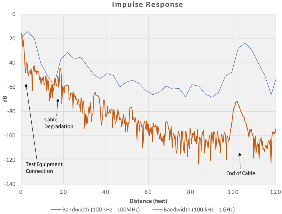
Figure 4.6. Example FDR impulse response data. Figure courtesy of AMS Corporation.
