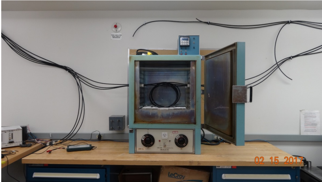
Figure 9.12. Accelerated aging experimental setup for heating 1.5 ft., 7.25 ft., and 10.5 ft. sections of three 100 ft. shielded three-conductor cables.
