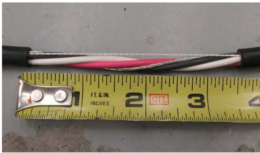
Figure 8.6. (left) Damaged 3.5 in. section at the halfway point of a 100 ft. three-conductor shielded 600V EPR cable; (right) corresponding ANSYS HFSS finite element model of damaged section.
