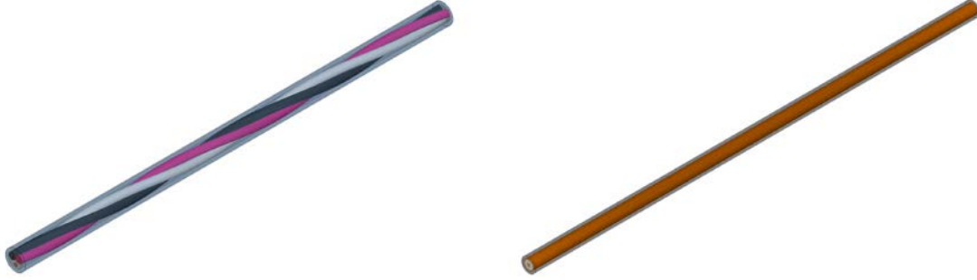
Figure 6.1. Example ANSYS HFSS simulation models representing segments of (left) three-conductor shielded cable and (right) coaxial cable.
