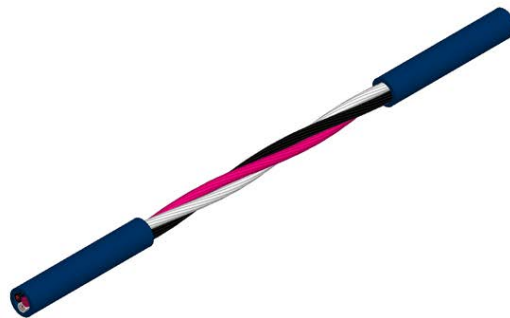
Figure 8.6. (left) Damaged 3.5 in. section at the halfway point of a 100 ft. three-conductor shielded 600V EPR cable; (right) corresponding ANSYS HFSS finite element model of damaged section.
