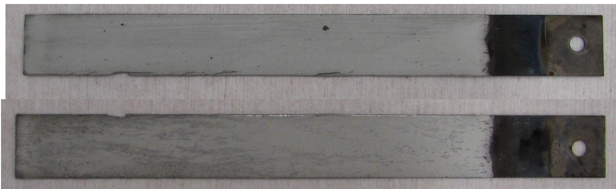
Figure 23. Foil Failed Foil (Q2E013) Post-Plating Images
