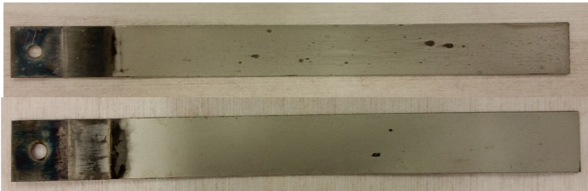
Figure 21. Failed Foil (Q1E045 (top), Q1E046 (bottom)) Post-Plating Images
