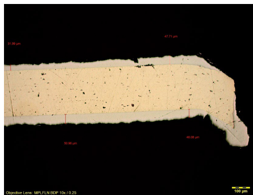
Figure 15. Q1E024 Showing Burr Effect on Plating
