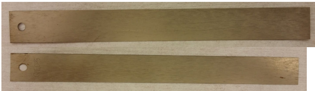
Figure 8. Receipt Inspection - Burr and Surface Defect
