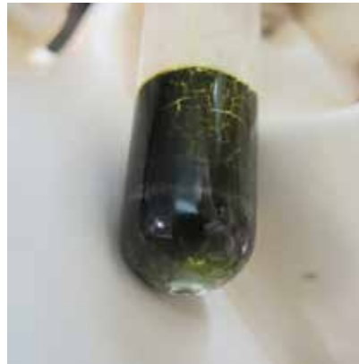
Plutonium oxide gel in a test tube produced while optimizing sol-gel chemistry.
