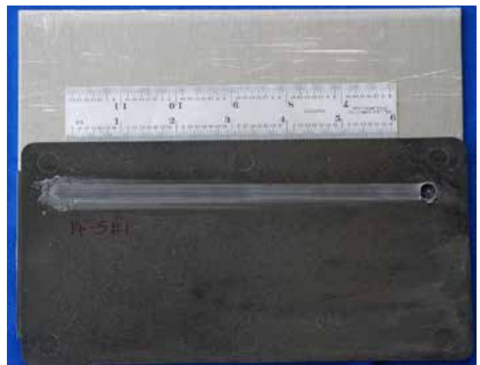
A representative FSST joint between carbon fiber reinforced nylon and aluminum sheet.
