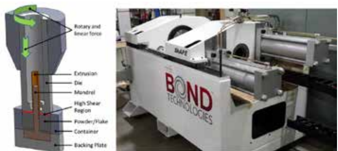
Schematic of ShAPE tooling and new state-of-the-art machine.
