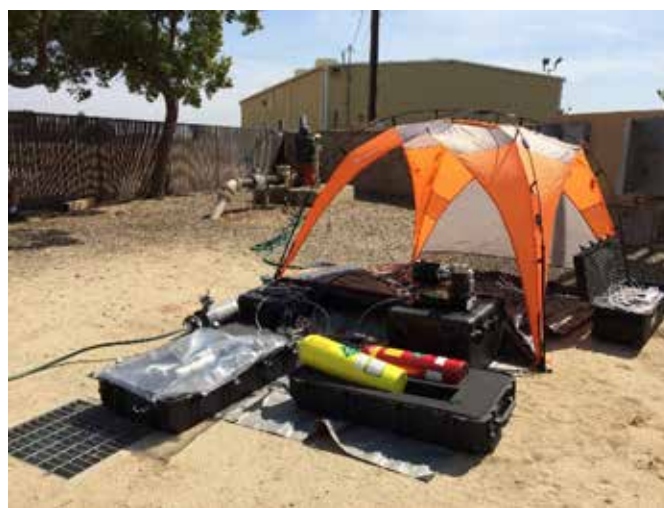
Degasification unit connected to a Tedlar® gas intermediate sampling bag and yellow/red SCUBA tanks used to collect the extracted gas.
