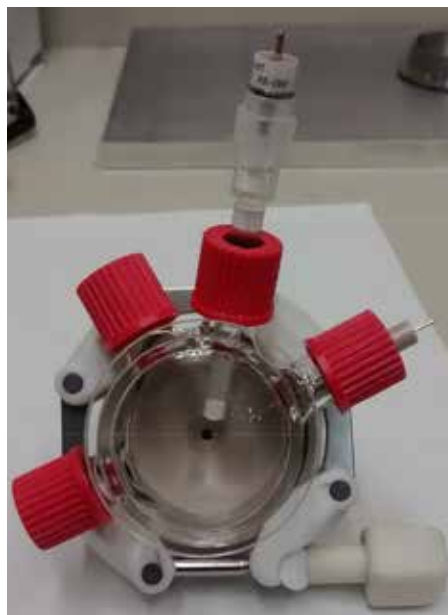
Photograph of custom-designed photoelectrochemical cell for measurement of oxide heterostructures grown by MBE.
