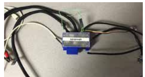
Sensor platform encased in 3D-printed enclosure with attached sensors.
