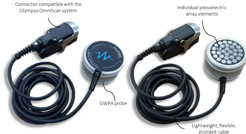
Figure 5 Photograph of a GWPA sensor that was used during the primary liner mockup inspection feasibility study
