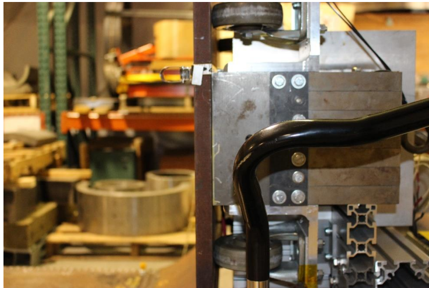
Figure 6.8. Side View of the Sensor in Place above the Knuckle for Examining the Surrogate Flaws Remotely
