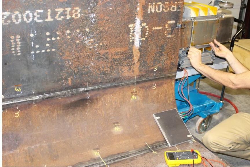
Figure 6.10. Meander Coil Being Replaced Between Examinations
