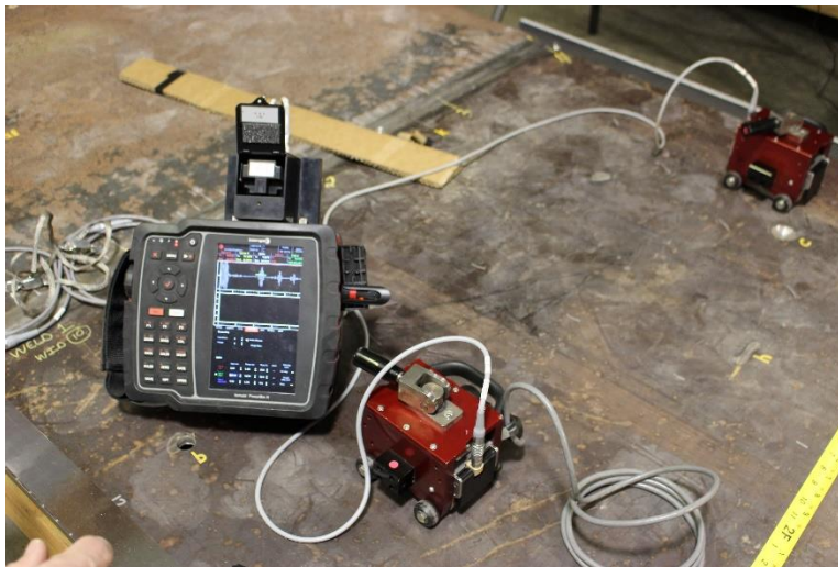
Figure 6.4. EMAT Pitch-Catch and Pulse-Echo Technique
