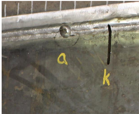
Figure 7.1. Photograph of Pit “a” (left) and Notch “k” (right) Located in the Transition Weld
