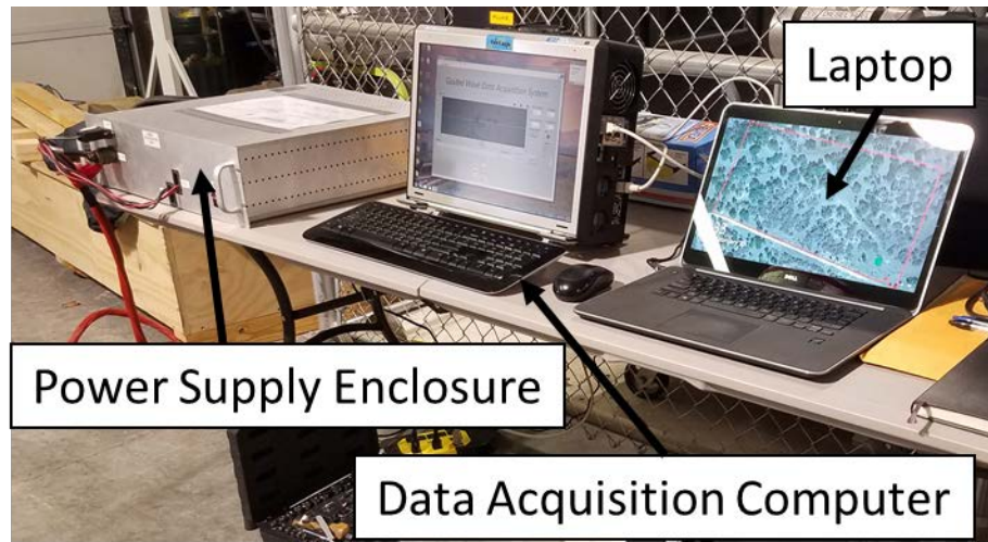
Figure 3. Photograph of umbilical cable (red cable) connected to the power supply enclosure (left-most box) and data acquisition computer with a LabVIEW application running. The laptop on the right is used for processing the data following the data acquisition process, but the processing could occur on the data acquisition computer if necessary.
