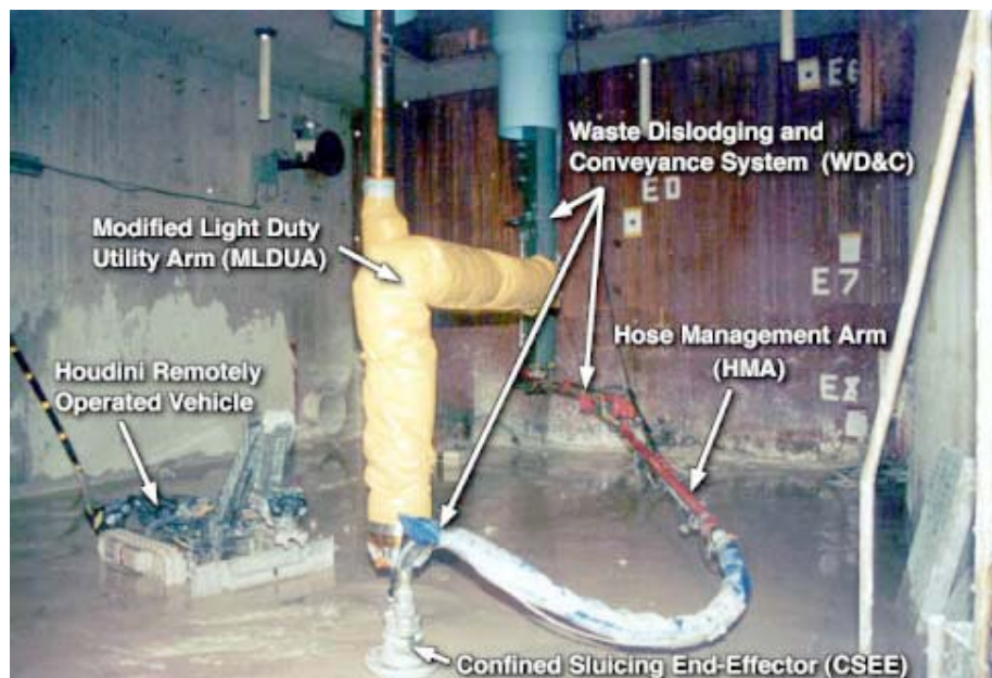
Figure 1.2. Confined Sluicing System Deployed in Tank W-3 at Oak Ridge Reservation (reproduced from Figure 4 of DOE/EM 1998)
