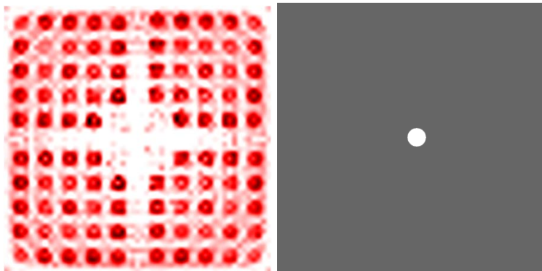
Figure 44. The reconstructed image from Figure 44 (left); a mask applied for identifying individual fuel rods in the image (right) (from Troeng 2004).
