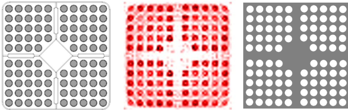
Figure 43. The cross section of the SVEA-96 fuel assembly (left), an example of a reconstructed image (middle), and the mask applied on the reconstructed images for deducing the position of the assembly in the measuring device (right).
