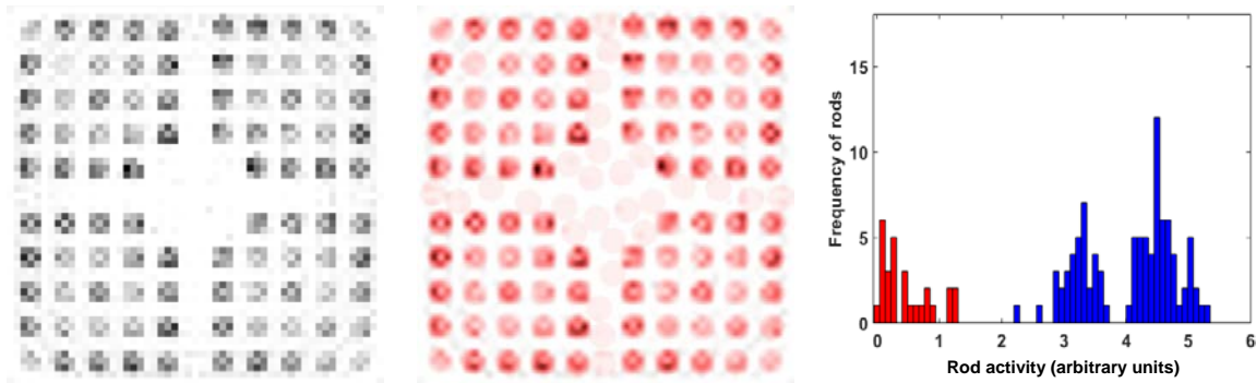
Figure 60. Reconstructed image of the ^{140}\text{Ba/La} distribution in the SVEA-96 fuel assembly that was measured using the PLUTO device in the Forsmark NPP in 2002 (left)(Jacobsson Svärd et al. 2005). The results of automated rod search in the reconstructed image, continuing until the whole image area is filled. Identified positions are overlaid in red over the reconstructed image (middle). A histogram of the rod activities extracted in the automated image analysis (right). The positions that correspond to actual fuel rods are marked with blue bars and non-rod positions are marked with red bars in the histogram.
