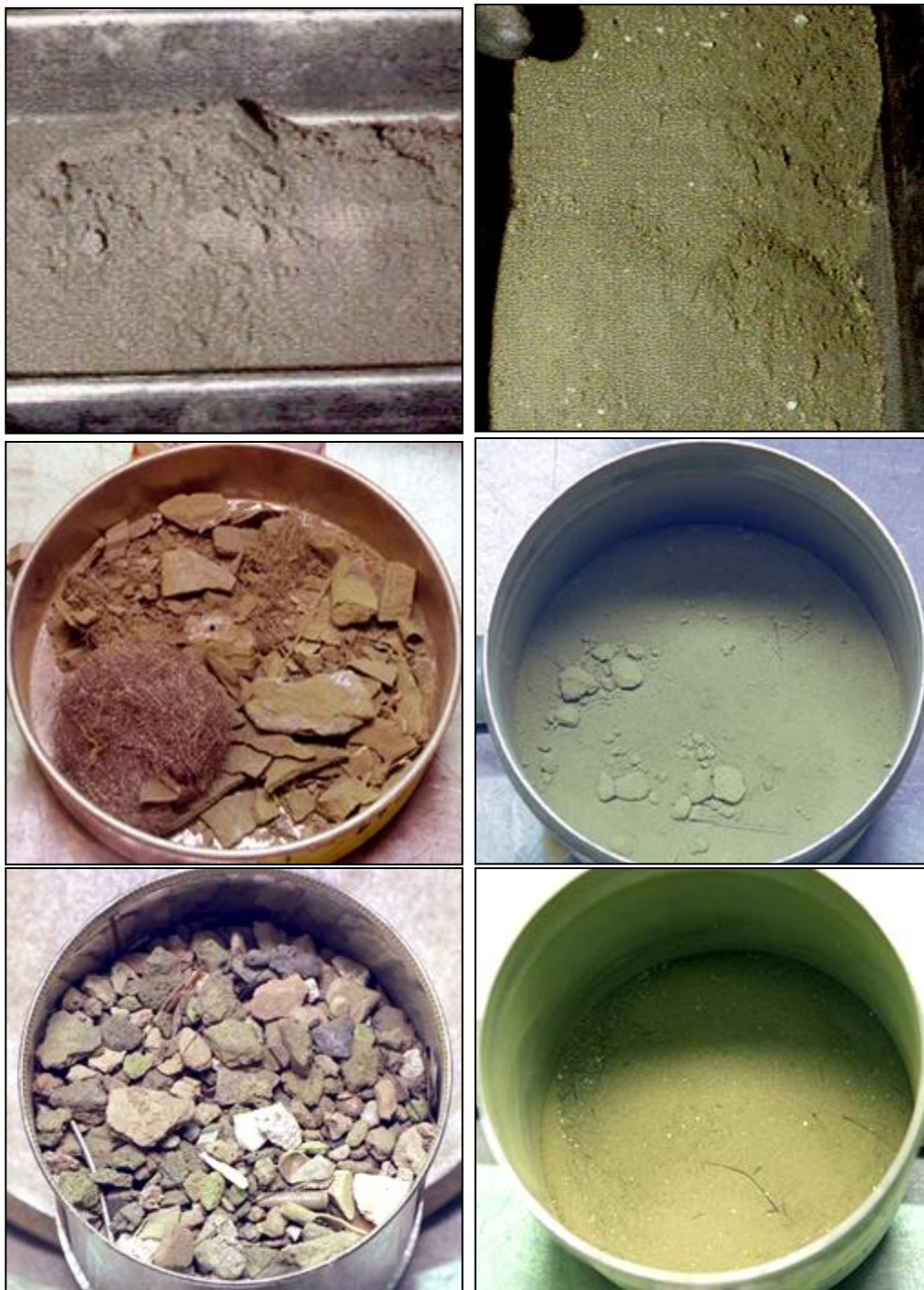
Figure 14. Plutonium Scrap from Rocky Flats. Top Left – Incinerator ash, ~16 wt% Pu. Top Right – Pulverized sand, slag & crucible, ~12 wt% Pu. Middle Left – Screenings from oxide, ~43 wt% Pu. Middle Right – Chloride-bearing oxide, ~72 wt% Pu. Bottom Left – Low purity oxide heel, ~54 wt% Pu. Bottom Right – “Pure oxide,” ~85 wt% Pu (note brush hairs and white particles)
