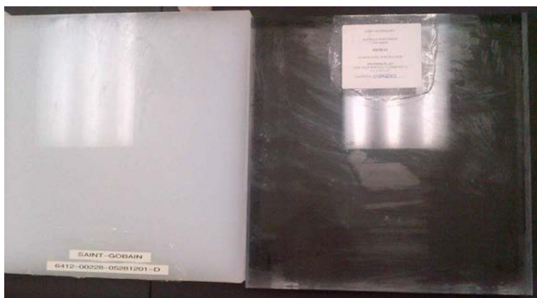
Figure 1.1. Internal fogging of PVT (left) after accelerated aging compared to unexposed PVT (right).
