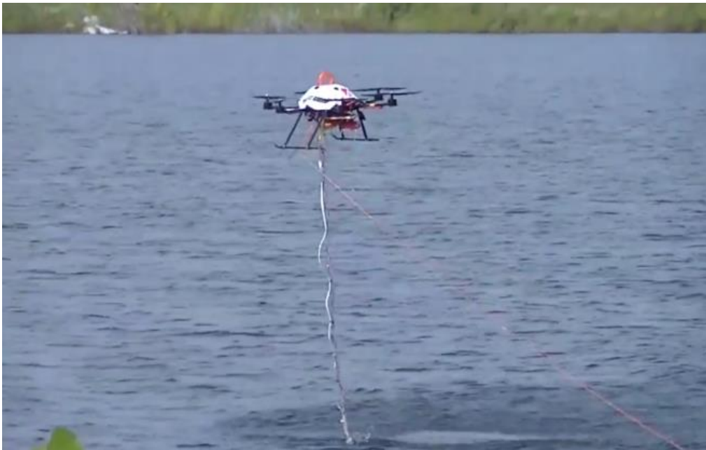
Figure 15) A water sampling aerial robot is being developed by the University of Nebraska, Lincoln – along with University of California Berkley - with funding from the U.S. Department of Agriculture.
