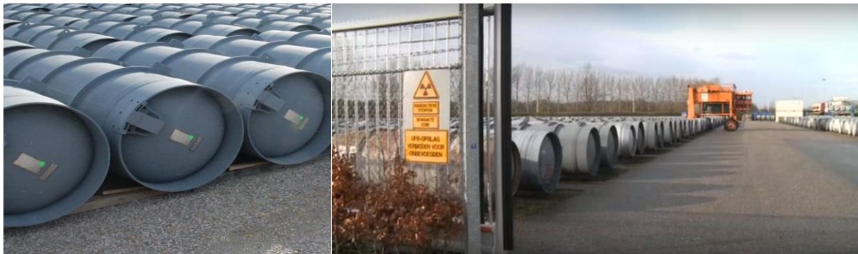
Figure 7) Examples of outdoor UF 6 container storage
