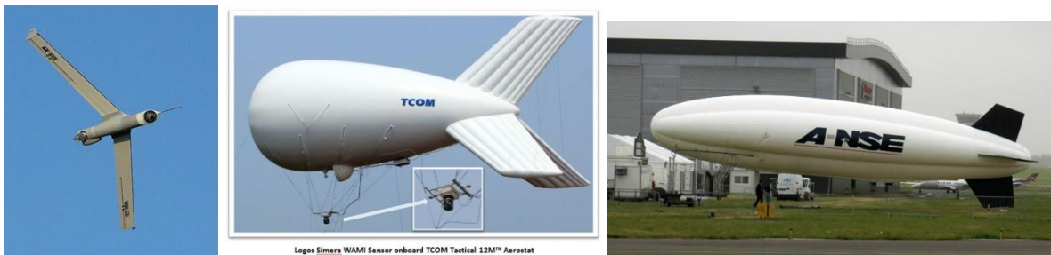
Figure 3) The Boeing "Scan Eagle" has a flight endurance of over 20 hours and carries advanced stabilized electro-optical and infrared camera. The TCOM aerostat with wide area camera is powered from the ground with a fiber optic cable.
