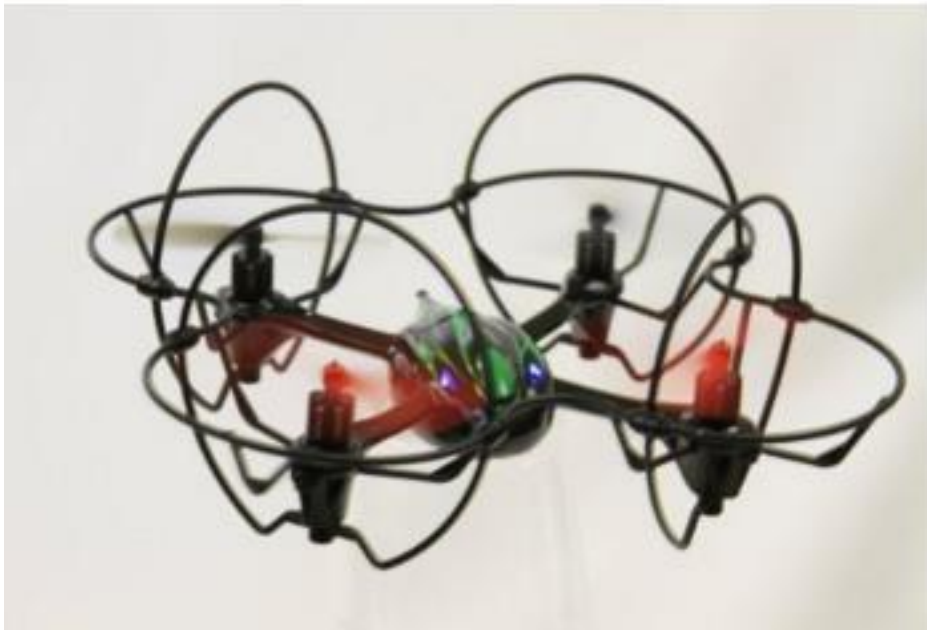
Figure 1) A small $40 quadcopter that could be modified and used to collect swipe samples from ceilings or walls
