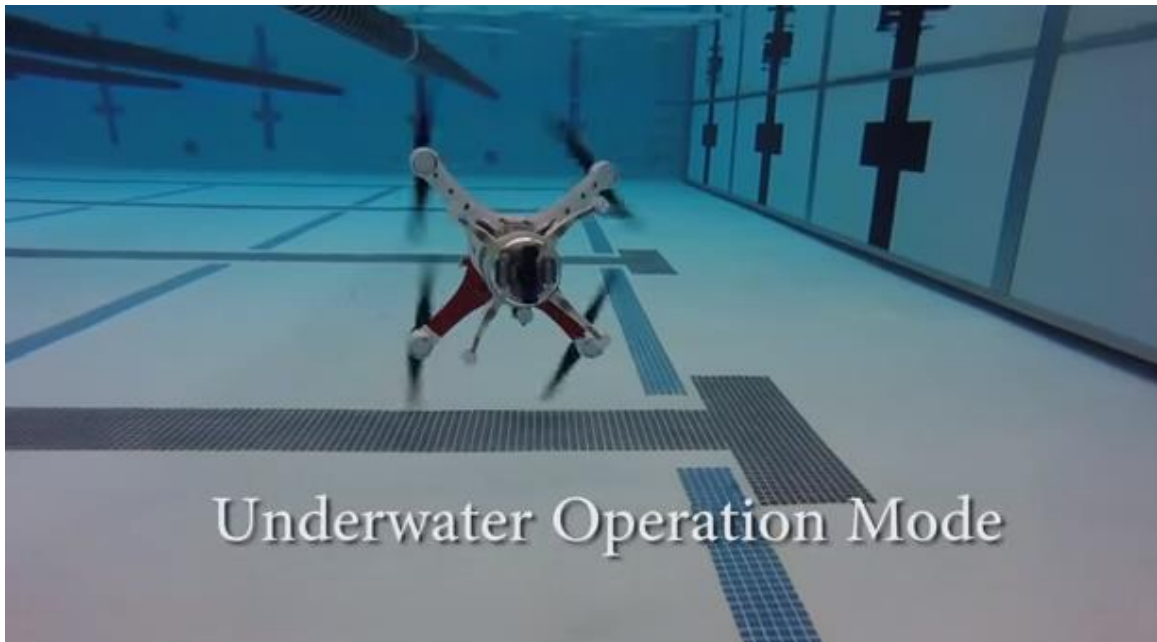
Figure 16) Oakland University "Loon" drone can endure stints of underwater operation, then rise to the surface and become airborne again.
