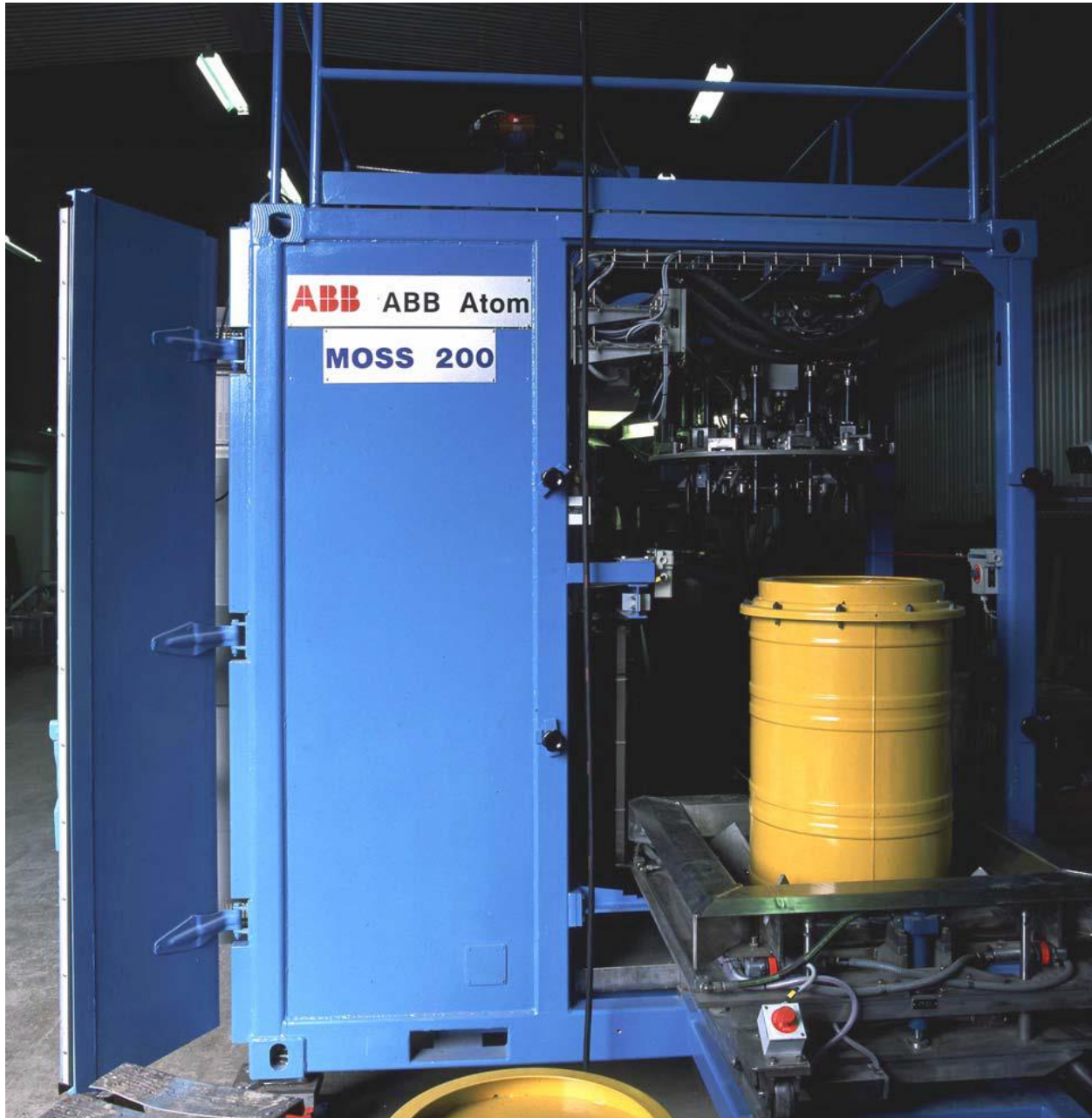
Figure 7.2. Photo of the MOSS unit with “lost-stirrer” to be utilized at Rossendorf (Gesser et al. 2000)
