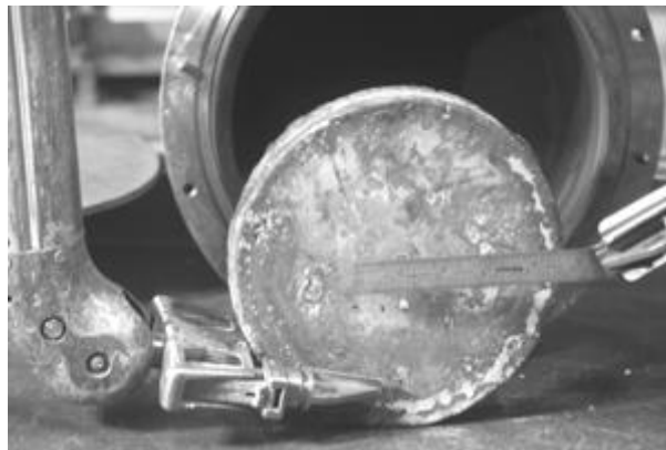
Figure 6.2. Photograph of Metal Waste Form Sample, from (Ebert 2005)
