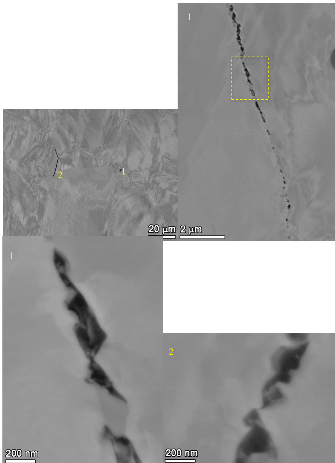
Figure 137. Apparent creep cracks in blunt notch specimen c672 cross-section slice #1 showing no evidence for corrosion or oxidation along the crack walls.
