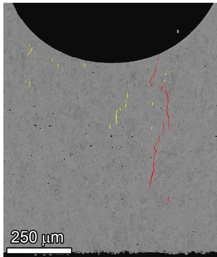
Figure 141. SEM-BSE image of C673 cross-section slice #4 showing cracks identified as SCC (red) and creep (yellow).
