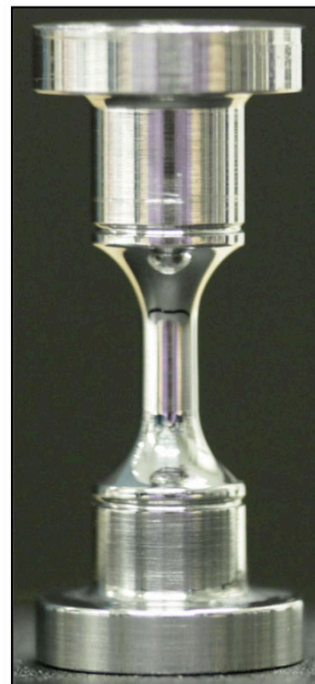
Figure 1. PNNL 1.2" tall SCC tensile initiation specimen.
