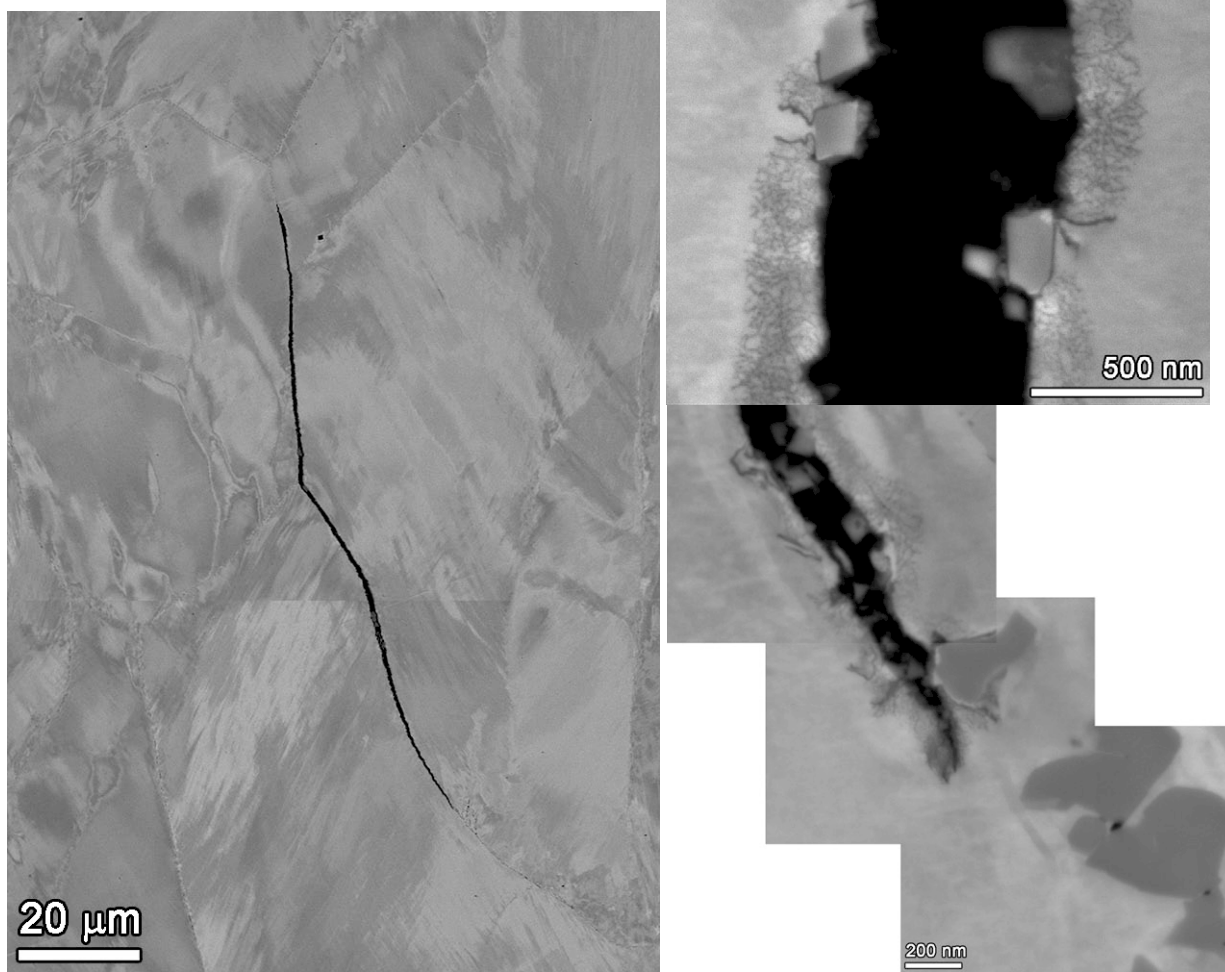
Figure 136. IGSCC crack in blunt notch specimen c672 cross-section slice #1 that clearly shows crack wall and crack tip corrosion.
