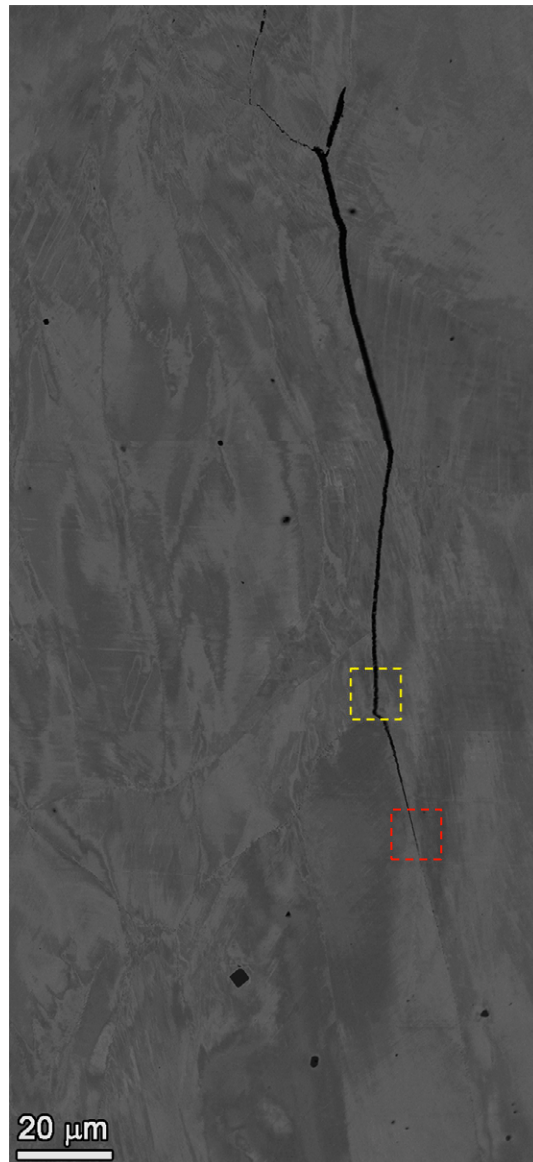
Figure 106. SEM-BSE micrograph of crack #1 in Figure 105. Note the red box near the visible crack tip and the yellow box further behind.
