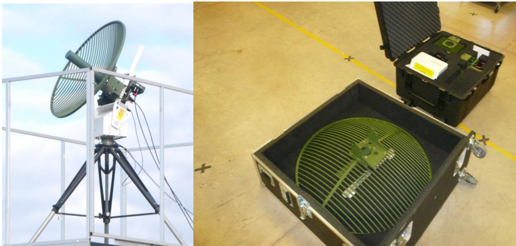
Figure 5.2. RAMS ground station antenna assembled and packed in transportable cases.
