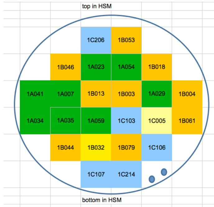
**Figure 8.2.** Fuel Assembly Loading and Identification Numbers for HSM-1
