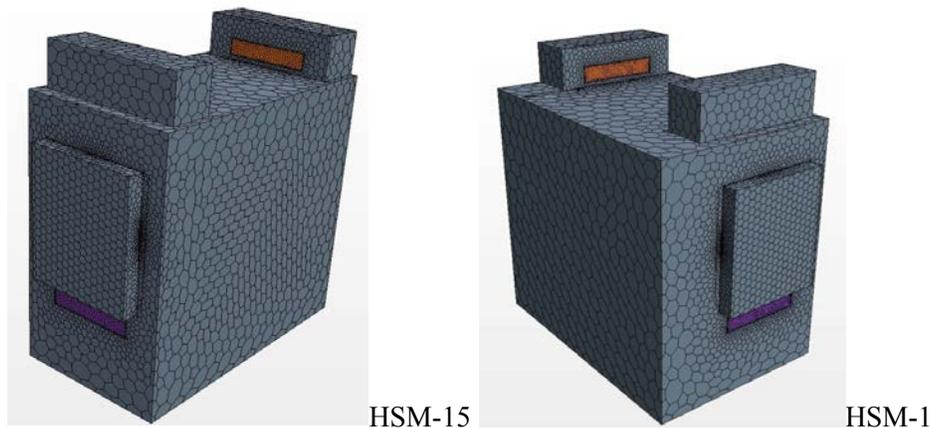
**Figure S.1.** Volume Mesh of HSM-15 Assembly: Exterior View
