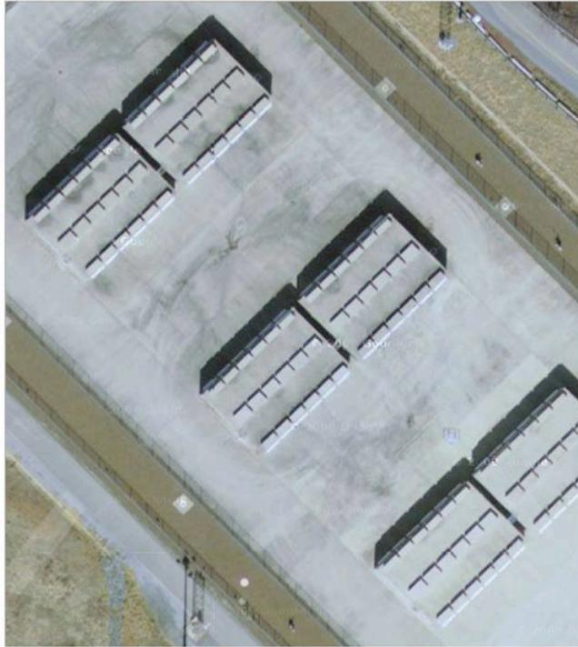
**Figure 1.1.** Aerial View of Calvert Cliffs Nuclear Power Station ISFSI, Showing Array of Six 2 x 6 Blocks of Storage Modules (Image U.S. Geologic Survey, Imagery Date: 2/28/2007, © 2011 Google)
