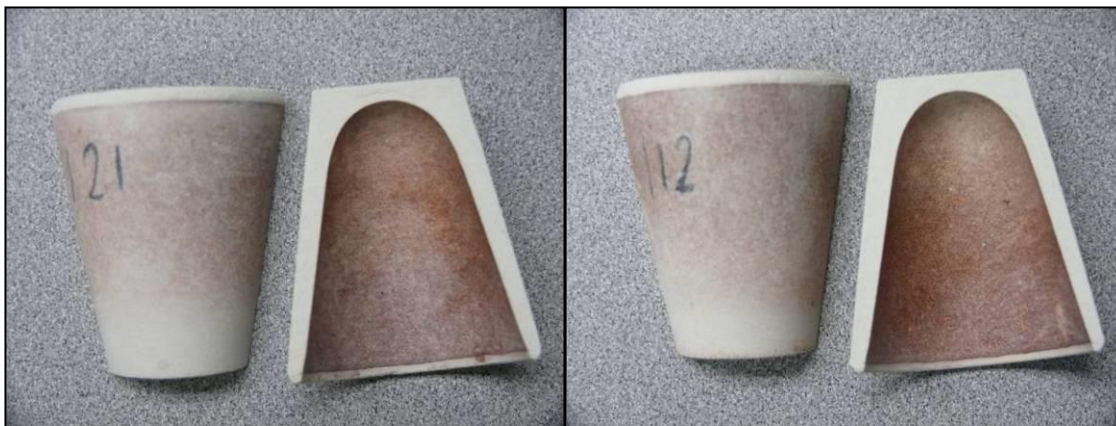
Figure 5.1. Cross-Sectioned Silica Crucible After Salt-Migration Tests; VSL BL Feed (left) and Al-Na-Limited Feed (right)
