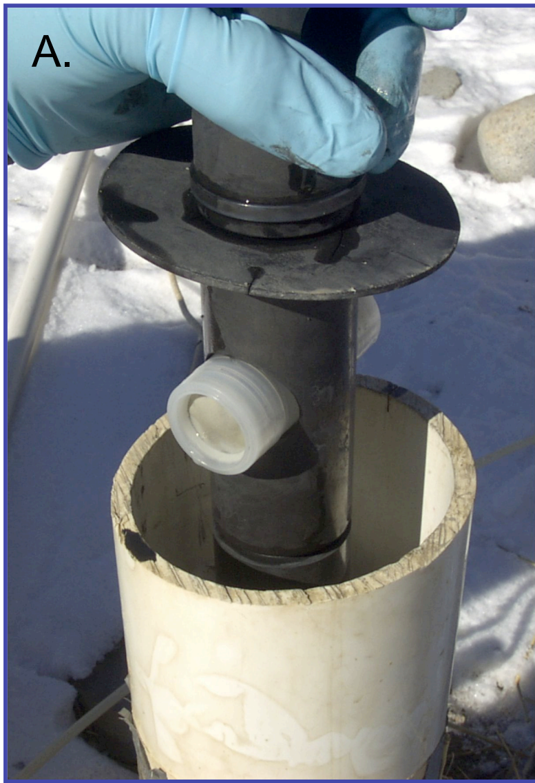
Figure 7. Passive multilevel samplers. A. Cell on support rod being lowered into monitoring well. B. MLS cells from a background well. C. MLS cells from a treatment zone well undergoing sulfate reduction.
