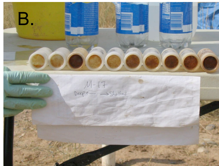
Figure 7. Passive multilevel samplers. A. Cell on support rod being lowered into monitoring well. B. MLS cells from a background well. C. MLS cells from a treatment zone well undergoing sulfate reduction.
