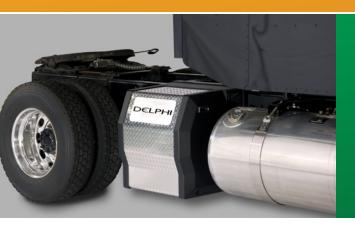
Today, long-haul truckers can power electronics without idling engines through use of auxiliary power units developed by PNNL and Delphi.
