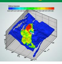
PNNL is using STOMP to model a recent DOE experiment in Alaska to improve understanding of how the guest-molecule exchange process works to produce methane hydrate gas.
